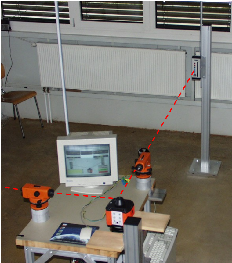
Figure 2: System for simultaneous adjustment of two axes (surveyor's table with PC and laser)
